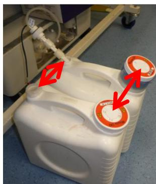
4. Place empty waste container on the Fluidics Cart and reconnect the 'quick connect' tube and **orange** coaxial cable to the Waste Port.
