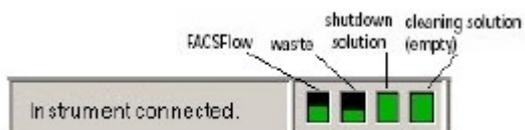
7. Check that the FACSFlow Cubitainer has sufficient sheath fluid in it and that the Waste Container is not full on the Fluidics Cart (see **Section 1.3. Infrequently Encountered Problems**).
